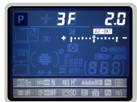
AEB settings on a Nikon D7000 (3 frames, at \pm 2 EV)
